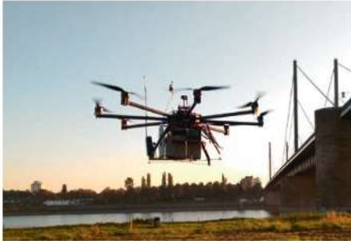
UMT drone (Oktocopter) for environmental measurements in Düsseldorf
